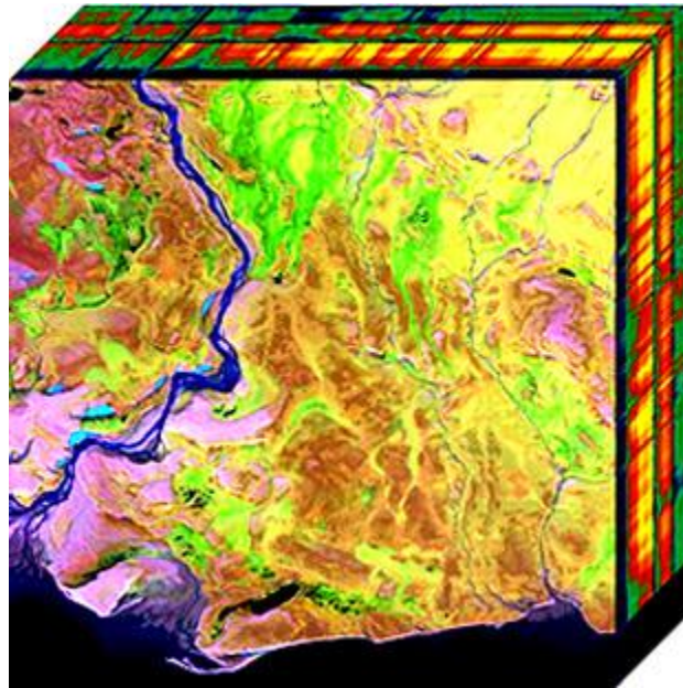
Two-dimensional projection of a hyperspectral cube
